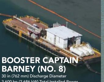
3,600 hp (2,686 kW) Total Installed Power
