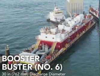
14,400 hp (10,742 kW) Total Installed Power
