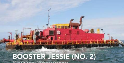
30 in (762 mm) Discharge Diameter 7,200 hp (5,371 kW) Total Installed Power
