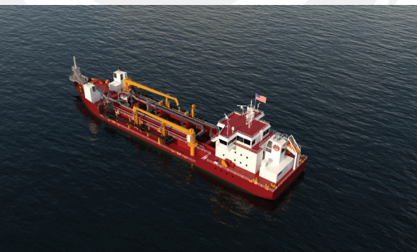
Illustration: GLDD's new build project, a 6,500 cubic yard capacity Trailing Suction Hopper Dredge.
