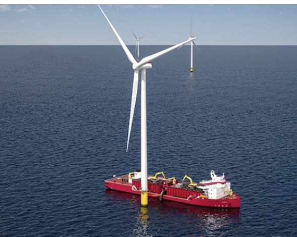
Illustration: GLDD's new build project, an inclined fall pipe vessel for subsea rock installation.
